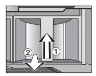
■ Lift the water container up and pull it forwards to remove it.
